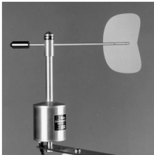
The small gap at North is filled to ensure smooth operation and a long service life. The precision ball-bearing races are corrosion-resistant and protected against the entry of moisture and dust.
