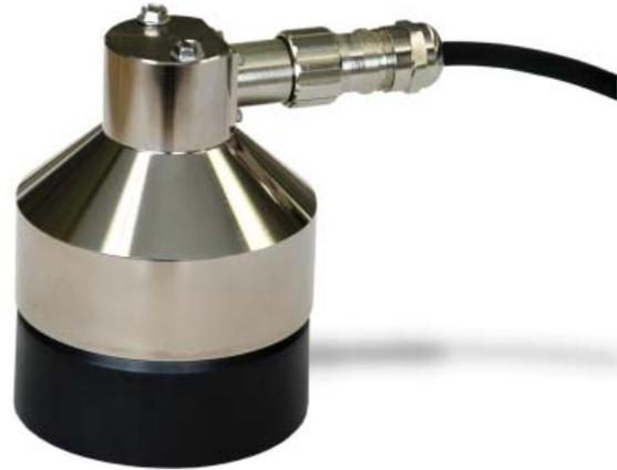
The SR50A was designed to meet the stringent requirements of measuring depths and uses a multiple echo processing algorithm to help ensure measurement reliability.
