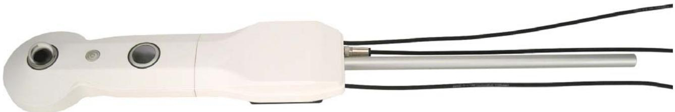
Above is a CNR4 net radiometer fitted with a CNF4 heater/ventilator unit. The CNF4 provides efficient air-flow over the domes.
