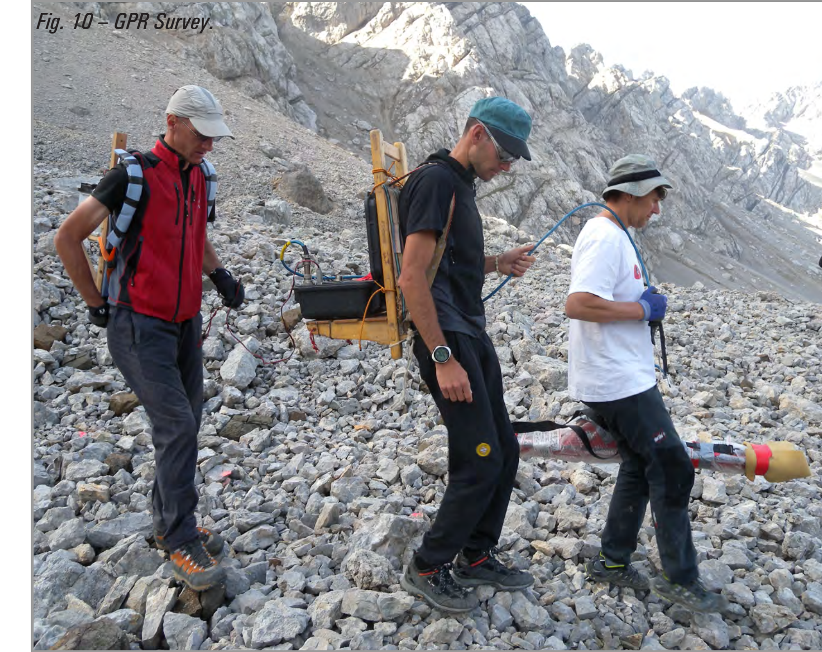
Fig. 10 – GPR Survey.
