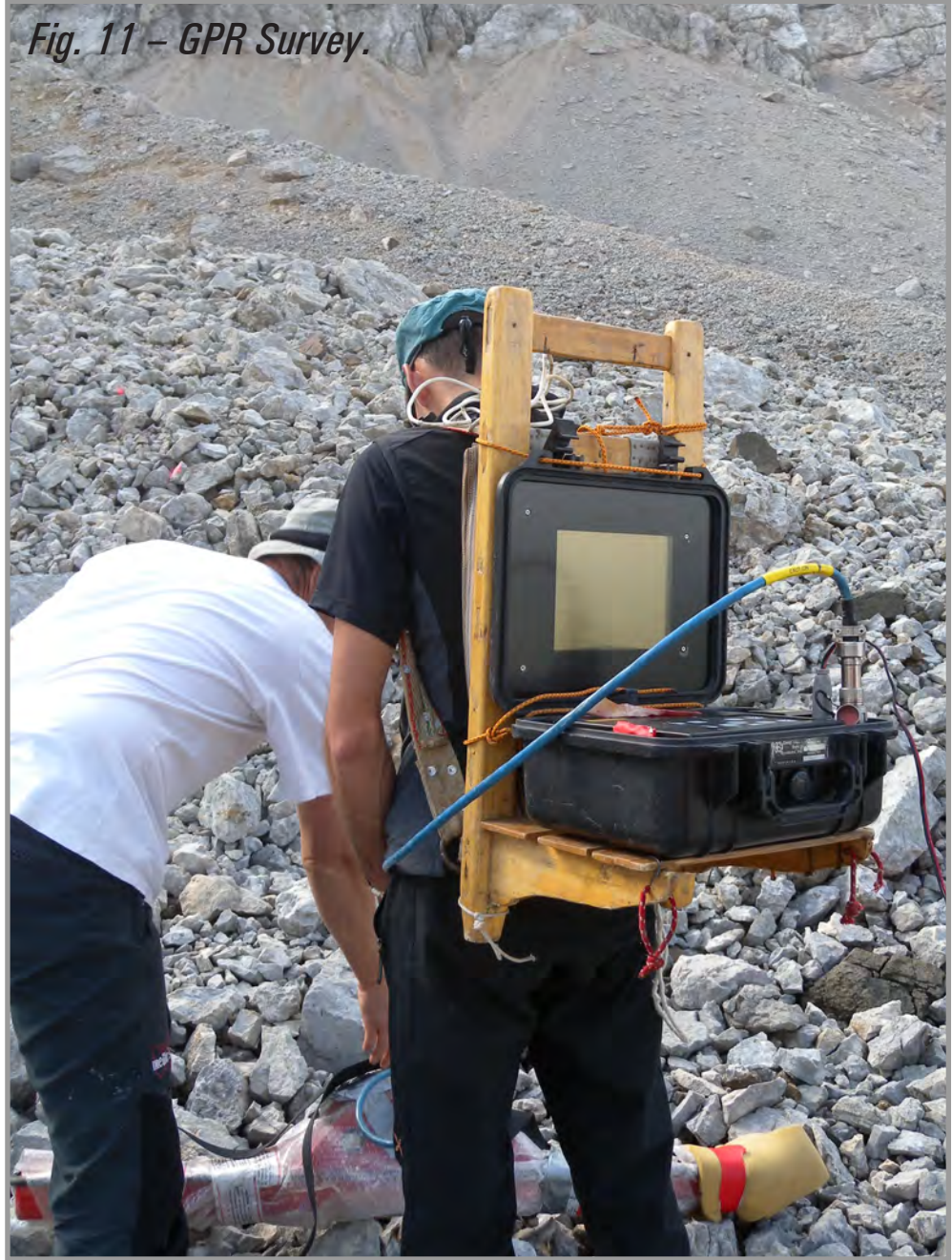
Fig. 11 – GPR Survey.
